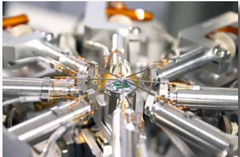
A completely encoded, eight positioner nanoprobe system (nProber).
