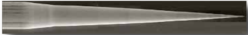
Composite SEM images (taken from the probe shaft to the probe tip). The slender taper angle allows for probing small geometries.
